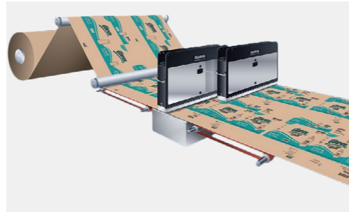
1. Package converting in a web process
