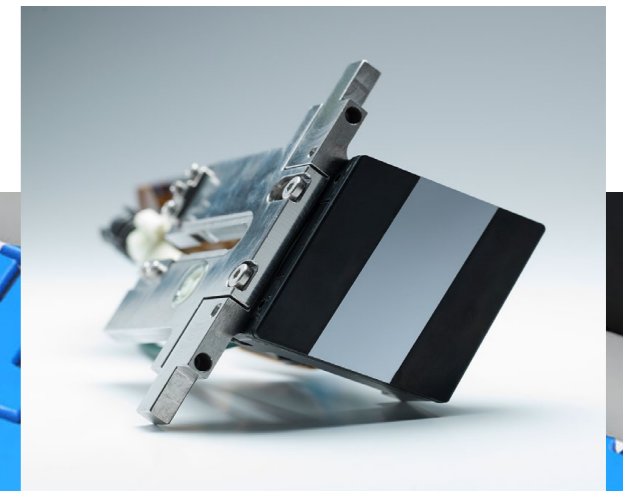
Samba printhead. Not visible to the naked eye, 2048 nozzles are contained in the silver coloured silicon chip which measures just 44 mm wide by 18 mm deep.
