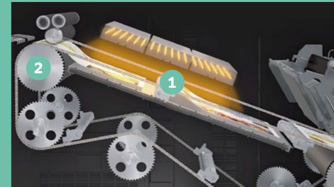
FIR low stress fuser 1 Far-infrared rays heating 2 Low pressure fuser roller
