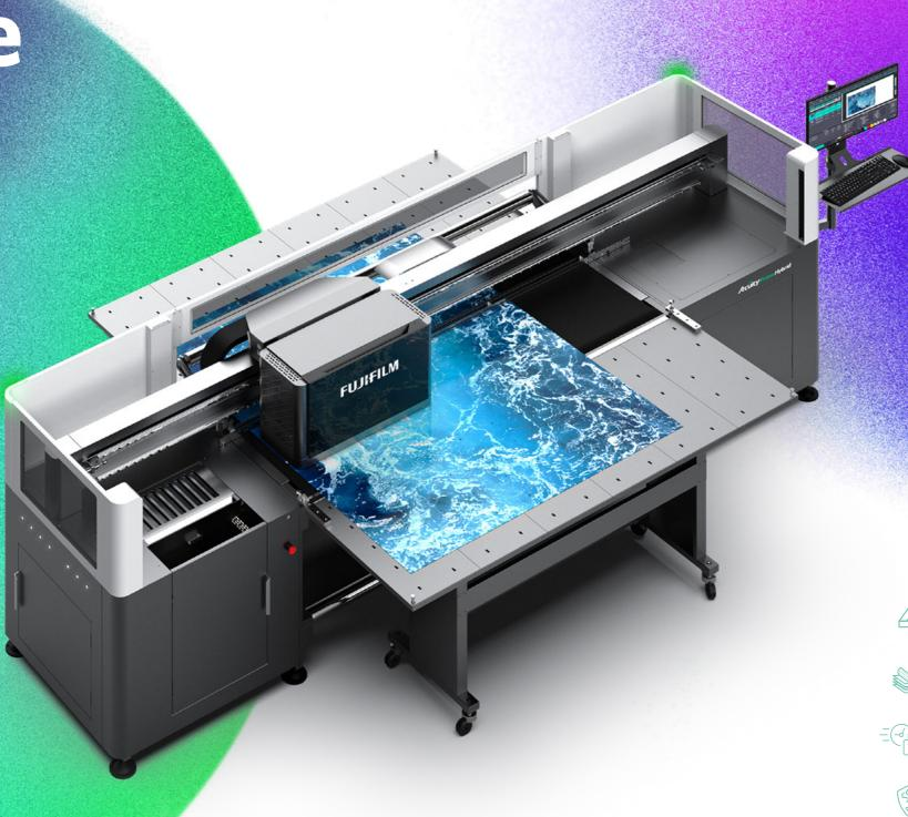
The Acuity Prime Hybrid can be configured with up to 7 channels, with CMYK as standard, and optional White, Clear and Primer, and produces stunning quality print, able to produce droplet sizes down to 7 pL. It handles flexible and rigid media up 51 mm thick, and roll media up to 2.1 m wide, and benefits from an ultra-reliable and long lasting air cooled LED UV curing system.
